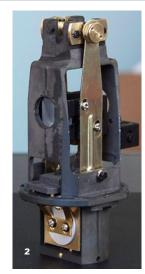
Laser filter for eyepiece
